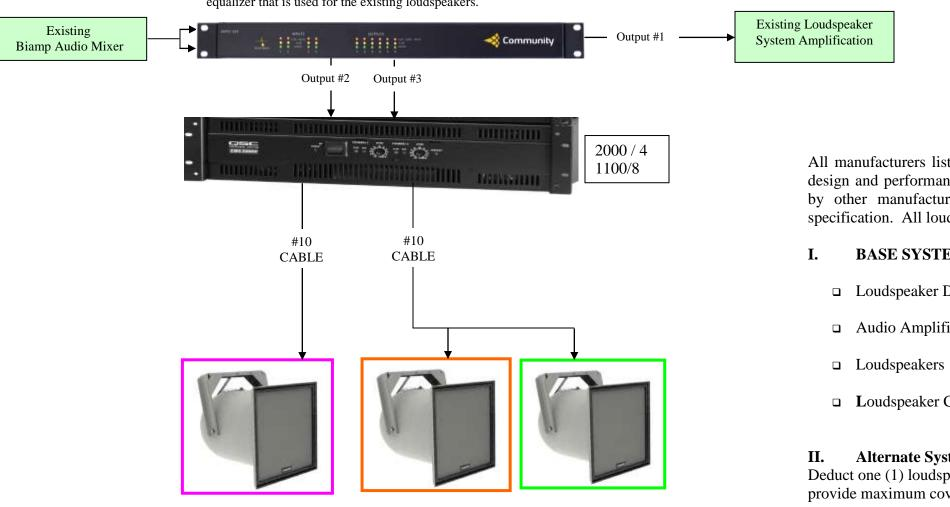
A portion of this loudspeaker DSP is to also replace the current dbx equalizer that is used for the existing loudspeakers.
