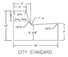
Answer: Yes, this is the detail. But this curb is being placed beside an existing road, so I can't say whether or not your curb machine will be able to place the curb. My experience with curb machines has been that the curb was placed before the road was built.
