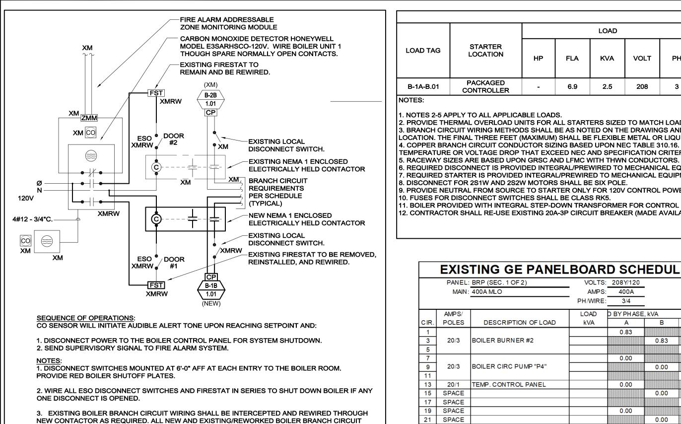
WIRING SHALL BE WIRED THROUGH NEW CONTACTOR AS REQUIRED TO ALLOW SYSTEM SHUTDOWN VIA CO DETECTION SYSTEM OR EMERGENCY SHUTOFF SWITCH/FIRESTAT.
