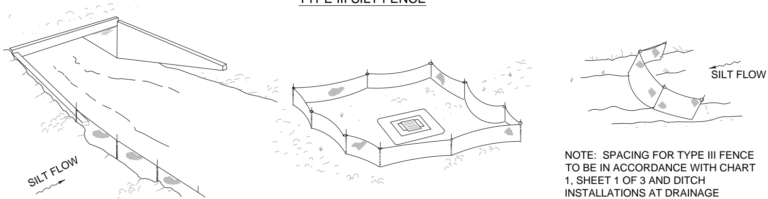
TYPE III SILT FENCE PROTECTION AROUND DITCH BOTTOM INLETS
