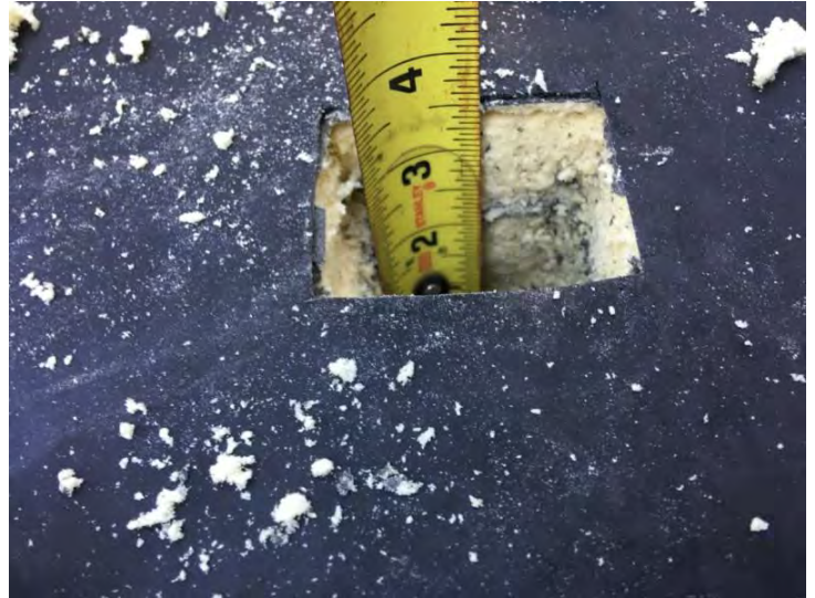
Test Cut Verified Dry Insulation from IR Scan
