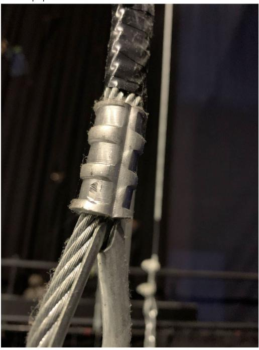
Termination points on all lines need to be adjusted to align with loft block positions.
